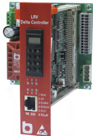
DELCON electronic control card on NTA-2
